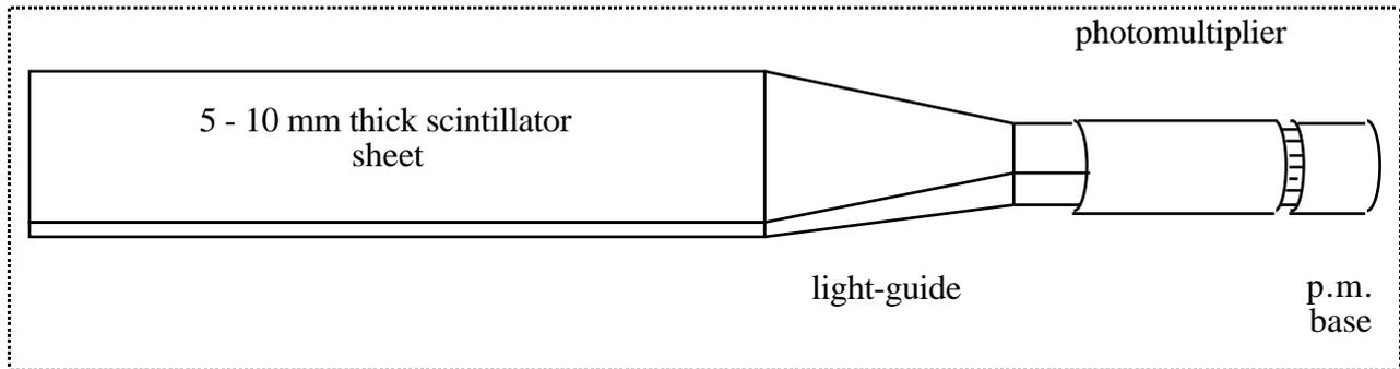
The scintillator may have an area of a few  $\text{cm}^2$  to  $\sim 1 \text{ m}^2$ , depending on the application. Light travels along the thin sheet undergoing many total internal reflections. Most light travels close to the critical angle, and the surfaces must be highly polished to avoid losses.
