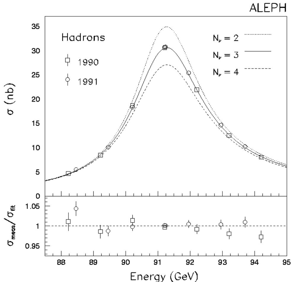
Fig. 7 Cross sections for  $e^+ e^- \rightarrow \text{hadrons}$  as a function of centre-of-mass energy. The Standard Model predictions for  $N_\nu = 2, 3$  and 4 are shown.
